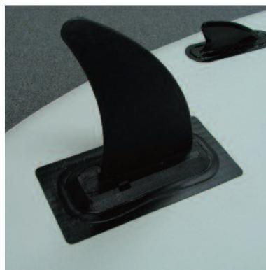
Slide the skeg into the skeg base underneath the stern. Then slide the key lock into the small gap in the base to lock it into place.
