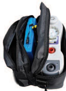
Keep the pump in its carry bag to make transportation easier and to protect the pump from sand which could jam it. The carry bag has compartments for the pump, battery hose.
