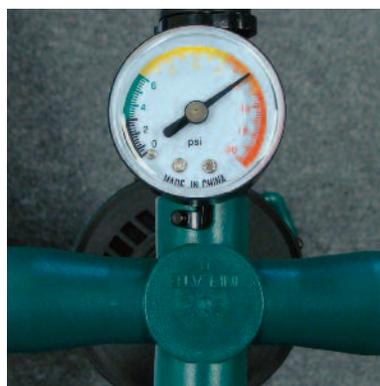
The pressure gauge will not begin to register until the board begins to get pressurized. Pump until the working pressure of between 12 and 14 psi is reached. **Do not exceed 15 PSI.**
