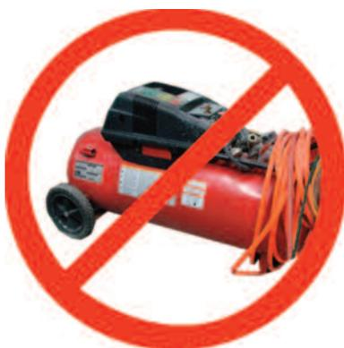
Air compressors that are designed for other uses like tire inflation (usually around 50 PSI) can easily harm your Sea Eagle. We only recommend using Sea Eagle pumps.
